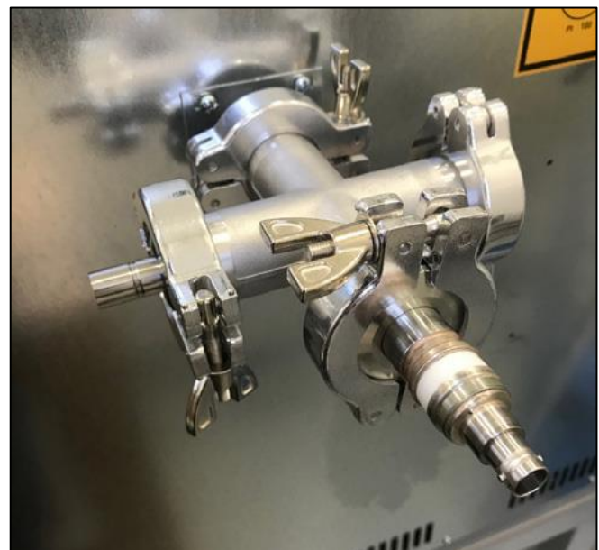
8. Figure - The picture of the Vacuum Bakeout Chamber electrical interfaces (outside)
