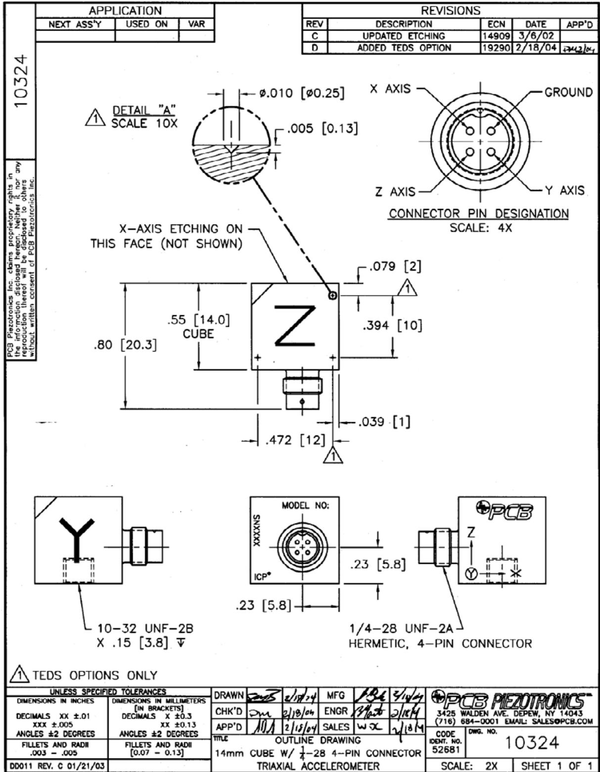
Figure 4 – Mechanical drawings of triaxial accelerometers and related interfaces (Witworth BSF 3/16"×32 or M6x0.75 course shall be provided on the tested item for fixture if needed)
