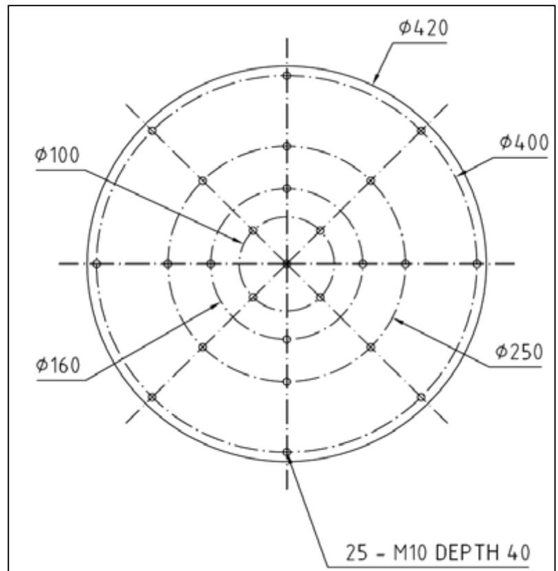
**Figure 3 – The shaker adapter, the fixing points are placed with distance given on the picture above (M10/40 screws can be used for fixing)**
