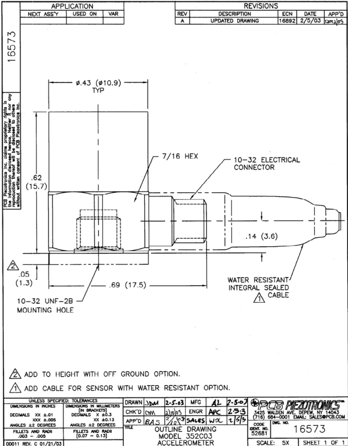
Figure 5 – Mechanical drawings of monoaxial accelerometers and related interfaces (Witworth BSF 3/16"x32 or M6x0.75 course shall be provided on the tested item for fixture if needed)
