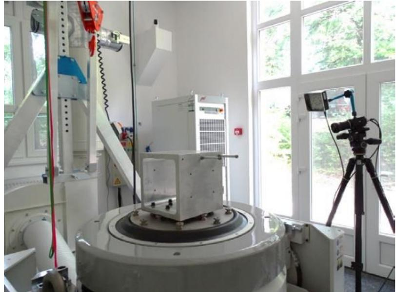
**Figure 2 – The picture of the Vibration Test System**
