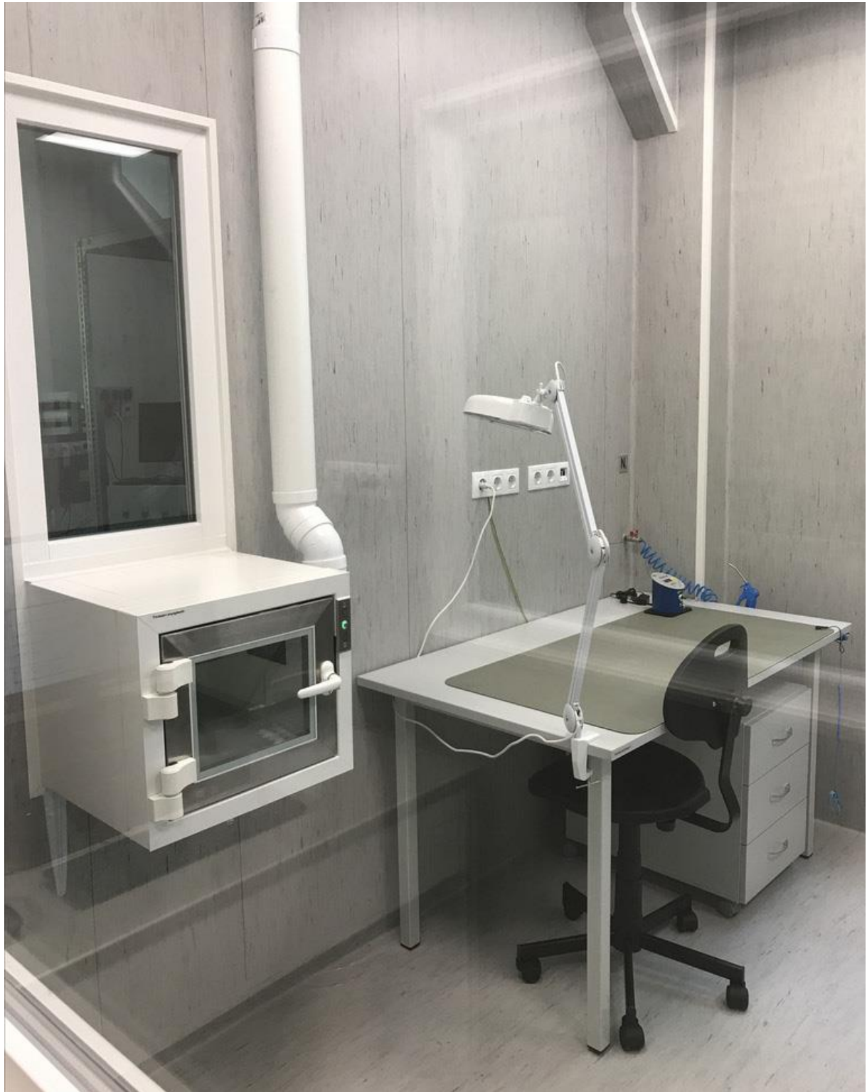
4. Figure – Cleanroom cleaning and assembly workstation with material airlock box
