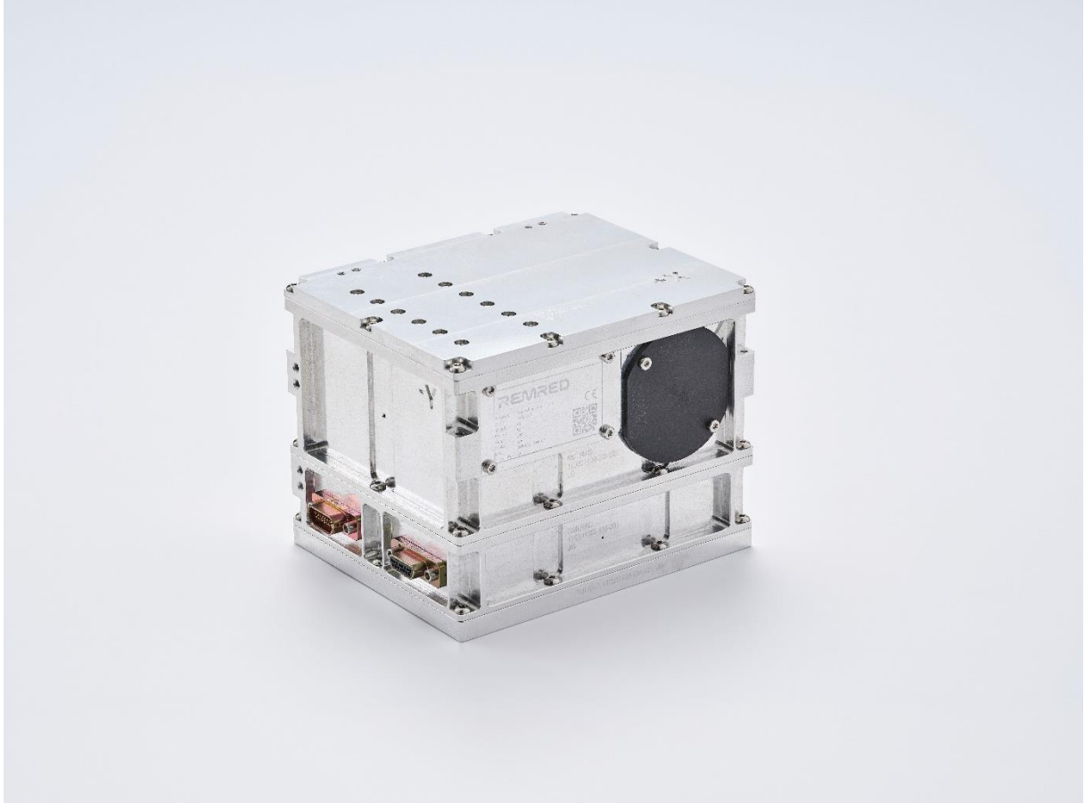
1. Figure – RML-RAD Space Radiation Monitor (1 st generation)
