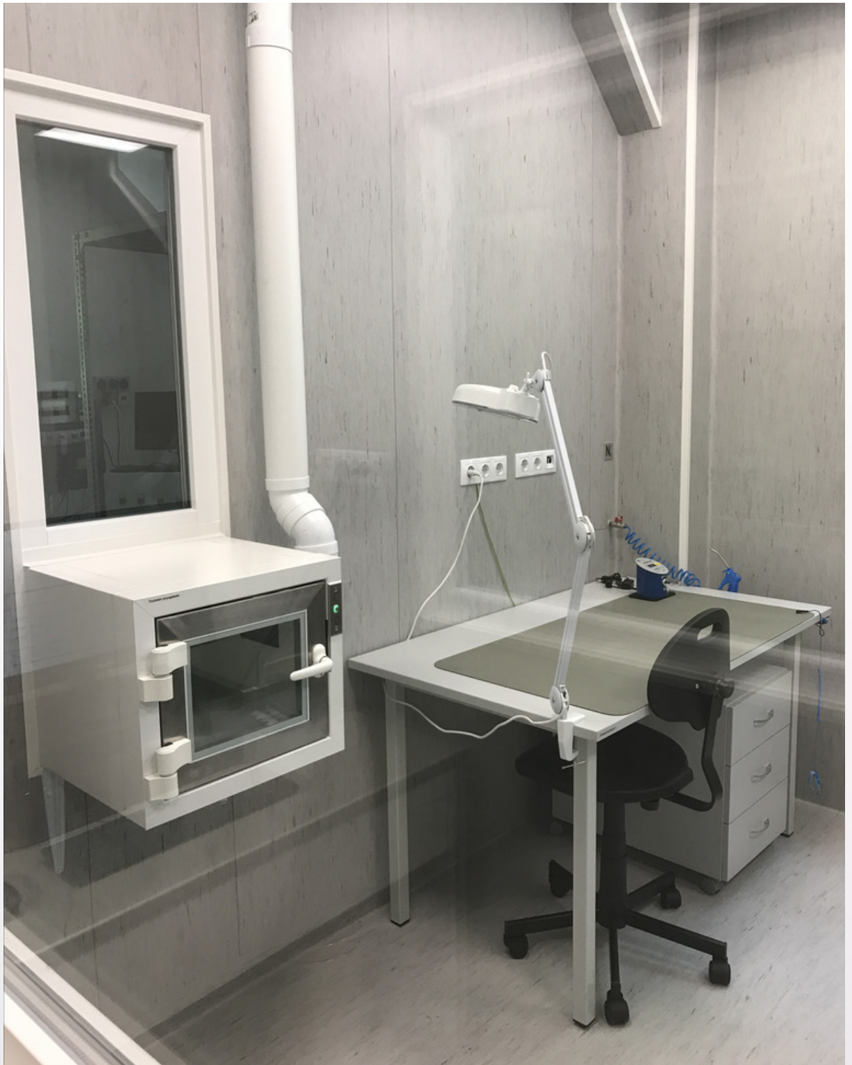
Figure 4 – Cleanroom cleaning and assembly workstation with material airlock box
